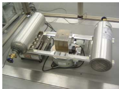
NMIJ Balance for gravimetric preparation of reference gas mixtures
