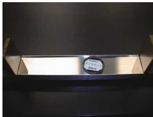
CVD diamond slider put on a stainless steel guide.
