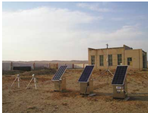
Photovoltaic System Operation Monitoring System at Sainshand, Mongolia. Irradiation, temperature, wind, ground albedo, and I-V characteristics of two types of PV modules are measured every ten minutes.
