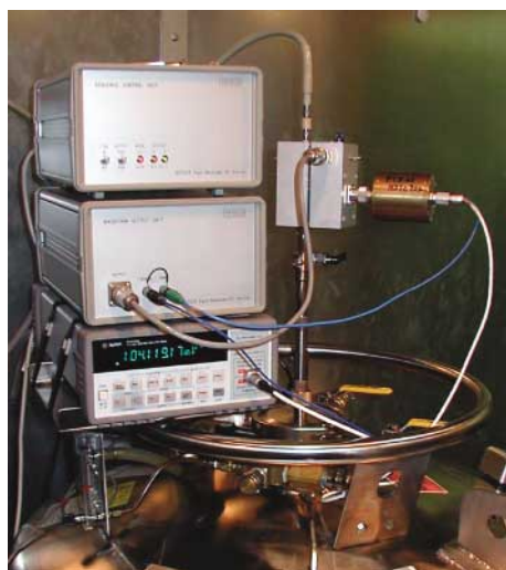
Measurement set-up for a Josephson-based Fast-Reversed DC
