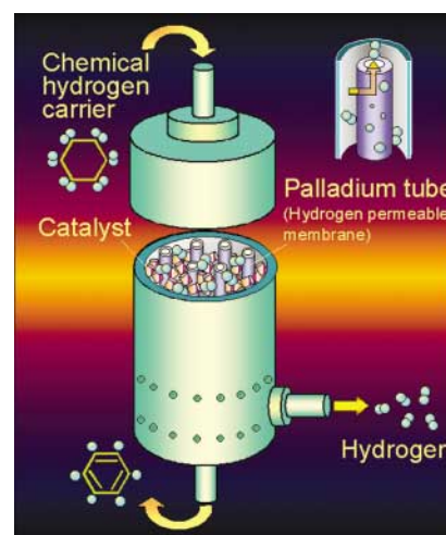
Recovery of pure hydrogen from chemical hydrogen carrier using a membrane reactor
