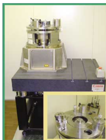
Automatic high precision calibration system for rotary encoder
