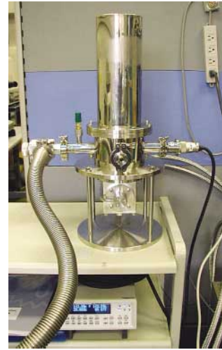
A photograph of a desktop Josephson voltage standard system
