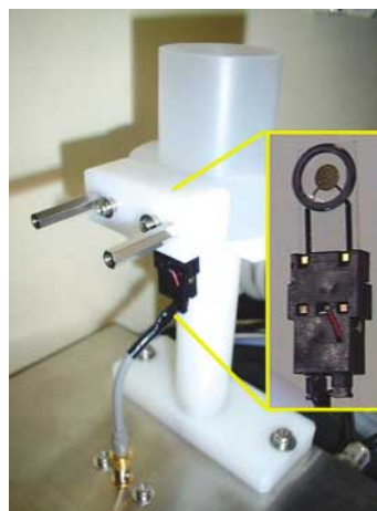
The appearance of quartz crystal microbalance and measurement cell
