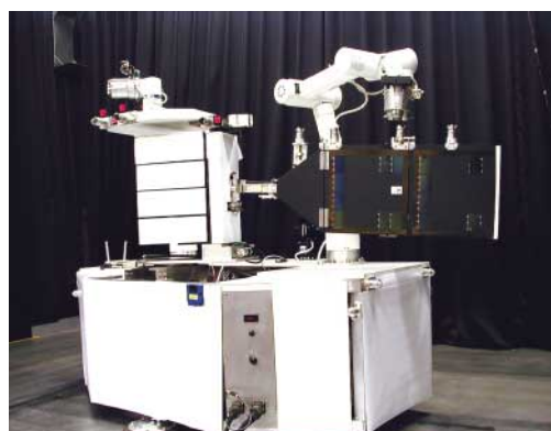
A Space Maintenance Robot on a Test Bed
