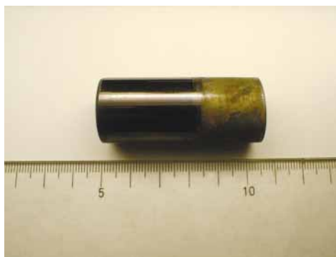
The surface of iron pipe with(left) and without(right) titanium oxide thin film after 3 week corrosion test in water
