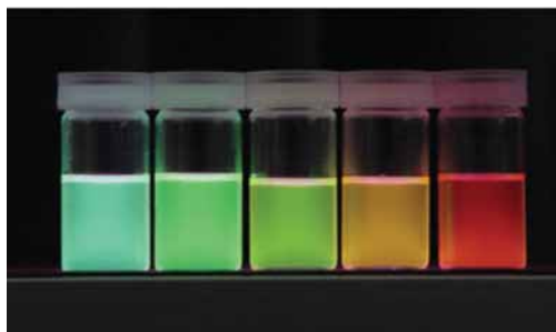
Fluorescence from nanoparticles of various diameters
