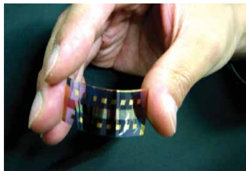
Organic thin film transistors prepared on a plastic substrate
