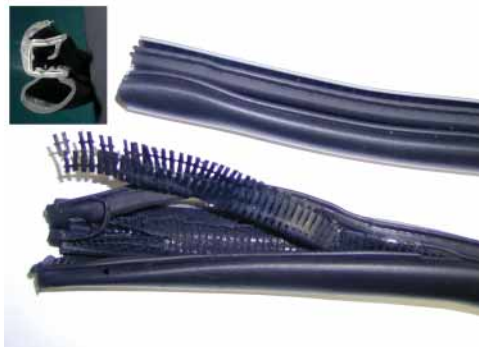
Separation of components in a car-window-seal composite by induction heating
