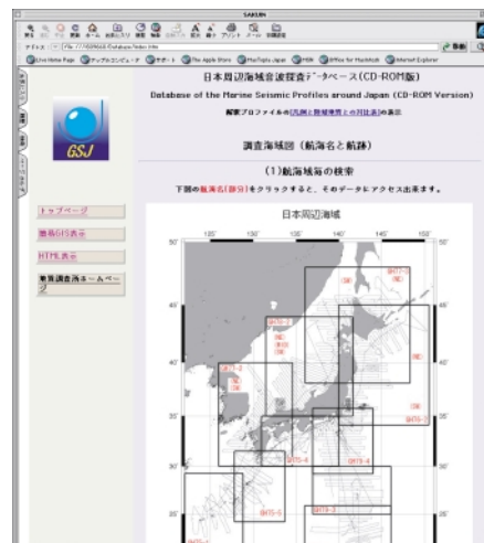
An example window shows an index map of seismic profiles around Japanese Islands. Each seismic profile can be searched and perused easily. Moreover, it is linked with the marine geological map, interpretation sections, etc.
