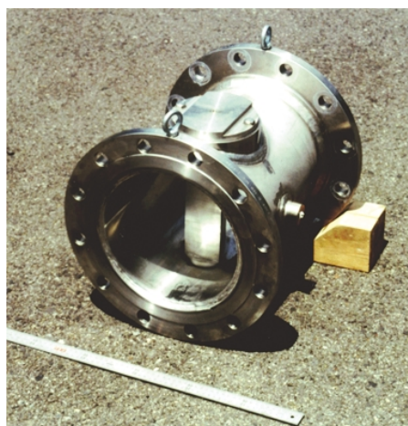
Photo of standardized vortex shedding flowmeter
