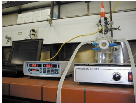
The QCM system for the detection of verotoxins produced by pathogenic bacteria: O-157.
