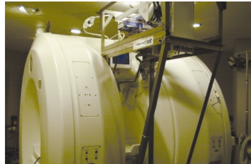
MR compatible surgical robot attached to an intraoperative MR scanner. It was the world's first fully MR compatible surgical robot.
