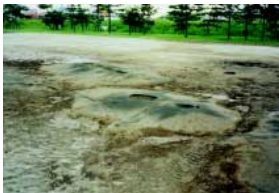
Sand blows on Oshamanbe, Hokkaido, after the 1993 Earthquake off the Southwest Coast of Hokkaido. The maximum diameter of the sand blows is about 2m
