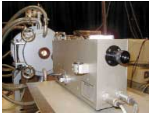
Eutectic point observation by radiation thermometer
