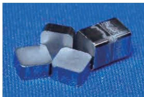
Development of post-neodymium magnets by low-oxygen powder metallurgy technology
