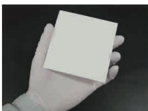
Electrolyte ceramic sheet for next generation all-solid-state batteries
